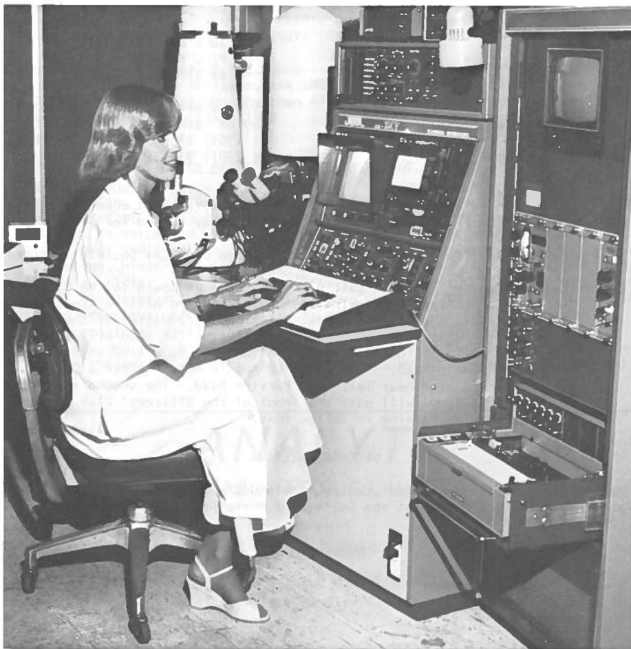
Civilian chemist and scanning electron microscope at Edgewood's Chemical Research and Development Center. Photo from the 67th anniversary special supplement to the APG News.
