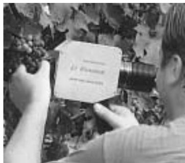
*Le Vigneron's* system combines physics and statistical analysis to perform its function. The first step in creating the applications was to acquire a database of the spectra of ripening grapes and known values for their brix, pH and TA. This database is the foundation of the statistical model that drives the predictions. As the model acquires more and more data points from the field, it will become more and more robust.
