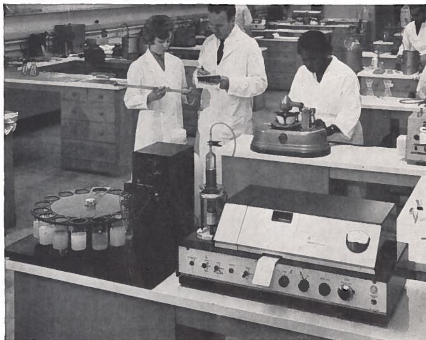
Titralyzer automatic titrator operates unattended. All a technician has to do is put new samples in turntable, keep reservoir filled with titrant.
