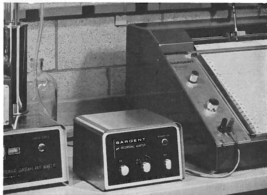
Actual laboratory application showing Sargent Constant Rate Burette with Magnetic Stirrer, pH RECORDING ADAPTER, and Model SR Recorder.
