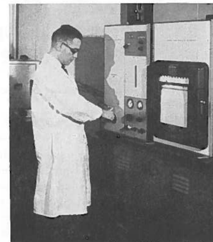
DR. ROBERT BLANKE, ASSISTANT TOXICOLOGIST, USING PERKIN — ELMER VAPOR FRACTOMETER IN RESEARCH ON IDENTIFICATION AND ESTIMATION OF VOLATILE POISONS
