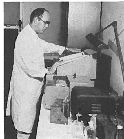
MARTIN KARST, SENIOR CHEMIST, USING BECKMAN DK—2 SPECTROPHOTOMETER FOR BARBITURATE ANALYSIS.
