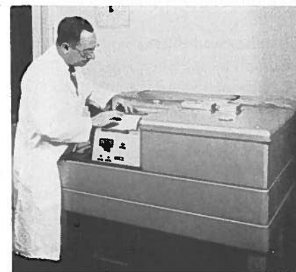
DR. HENRY C. FREIMUTH, TOXICOLOGIST, USING BAIRD INFRA RED SPECTROPHOTOMETER TO IDENTIFY ORGANIC POISON EXTRACTED FROM TISSUE.
